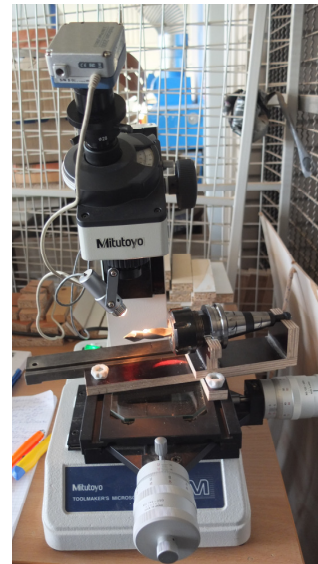
Fig. 3. Determining the size of the wear indicator of the external corner ( W ) of the drill
